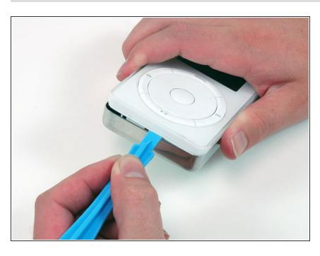
Work around the corner of the iPod and release the two tabs holding the iPod together near the dock connector.
