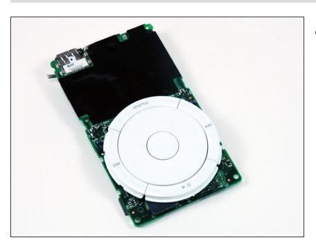
Logic board & attached scroll wheel remain.
