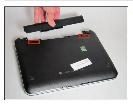
Remove battery by pushing the two tabs and pulling the battery outwards slowly but firmly.
