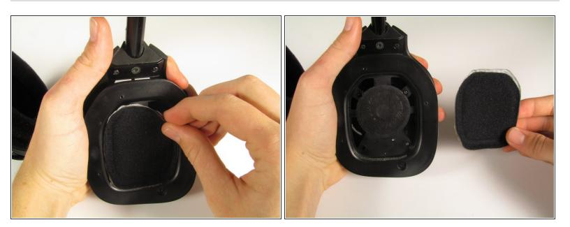
Using either your fingers or a plastic opening tool, pry off the speaker cover.
