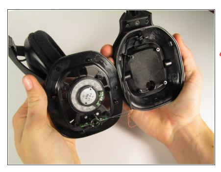
• Remove the housing to reveal the speaker.
