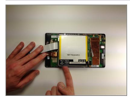
• Remove the battery from your device by applying pressure at the base of the battery and lifting it out.
