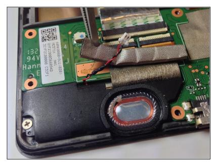
• Slowly peel off the EMI gasket over the ribbon cable assembly. This will expose the ribbon cable which can be removed from the connectors.
