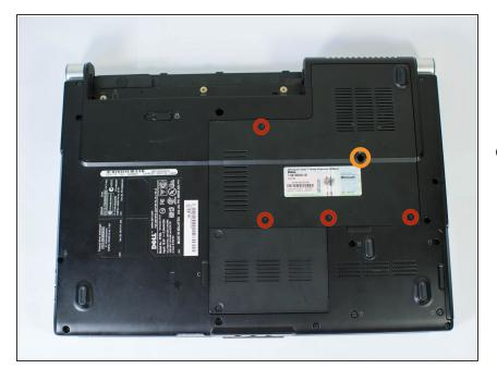
Unscrew the four Phillips #1 screws holding down the back panel. Then remove one 5.8mm Phillips #1
