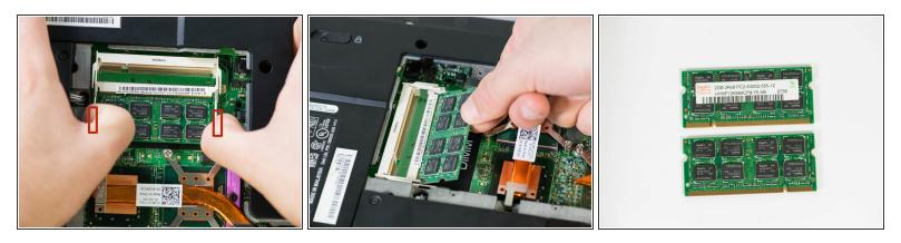
Push out on the second set of metal tabs to release and remove the lower RAM chip.
