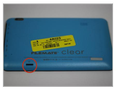
Locate the hole on the bottom left hand side of the backplate.
