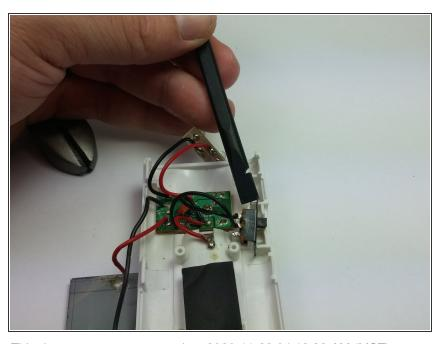
Using a spudger carefully pry switch from housing.
