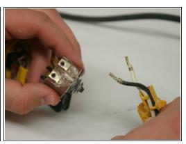
Using the J-1 screwdriver, unscrew the power cord wires from the red switch box (located in the back of the grinder).
