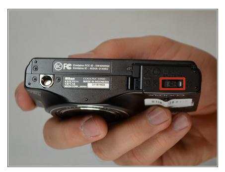
Locate the battery hatch on the bottom of the camera and slide the latch to the left.
