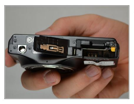
Swing open the battery door to expose the battery compartment.
