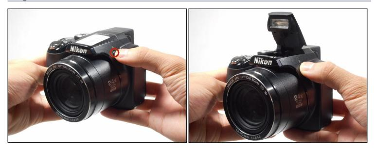
Press the button located on the top-right side of the camera's body to open the flash compartment.
