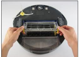
Push down on the two yellow tabs, and pull open the brush gate gently
