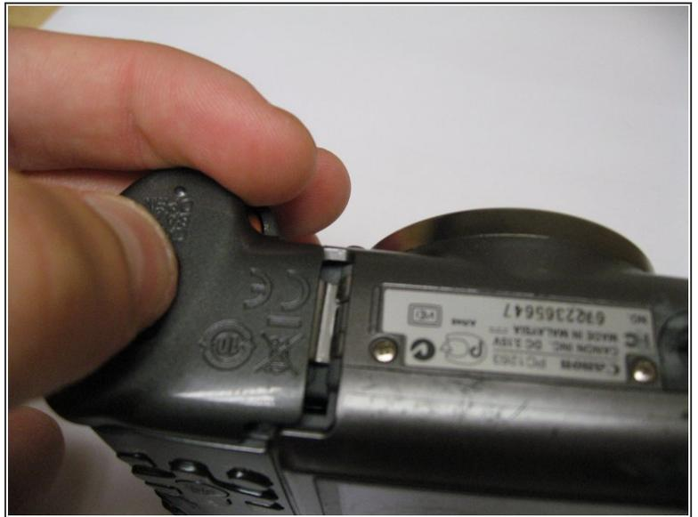
**i** The battery hatch is on the bottom of the camera.
