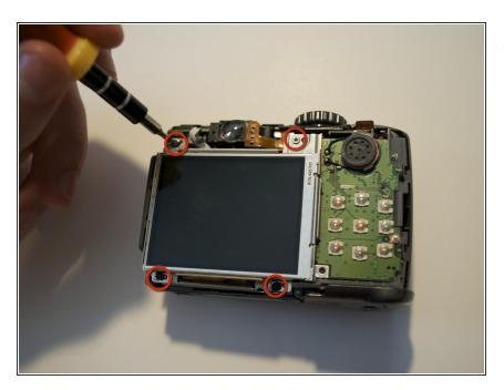
Remove the four screws near the corners of the LCD using a Phillips #00 screwdriver.
