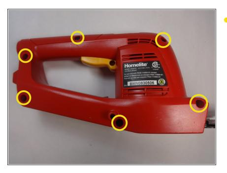
Remove the six 15 mm screws from the shear using a Phillips #2 screwdriver.
