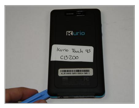
Make sure to open the back cover easily using the plastic opening tool.
