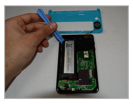
Use the plastic opener to remove the battery.
