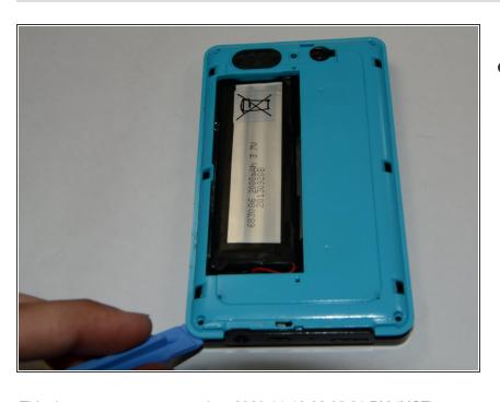
After you remove your four 5mm Philips screws use your plastic opening tool to help you open the plastic cover of your device.
