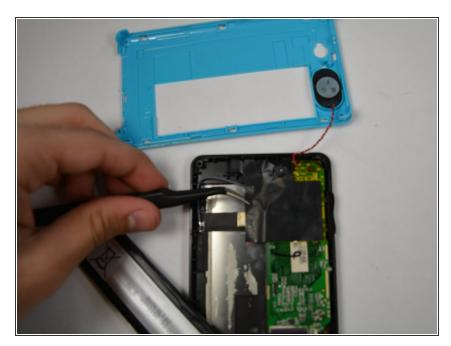
Use tweezers to remove the black tape that is attached to the motherboard.
