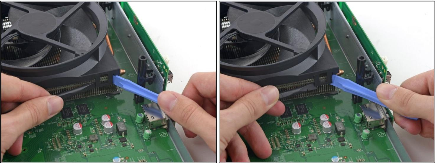
ⓘ The fan is held onto the heat sink with four sturdy plastic clips. By prying the two exposed clips up out of their channel in the heat sink, you'll be able to tilt the fan up and off of the heat sink.
