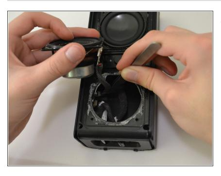
Firmly pull on the end of the ribbon cable to disconnect the speaker from the motherboard.
