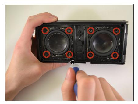
Using a #000 Phillips Screwdriver, unscrew the four 0.8 cm Philips screws from each corner of the speaker you are replacing (eight 0.8 Philips screws total).
