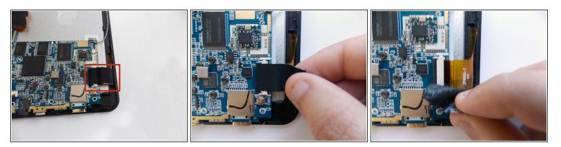
• Remove the black tape covering one of the screen power cables.
