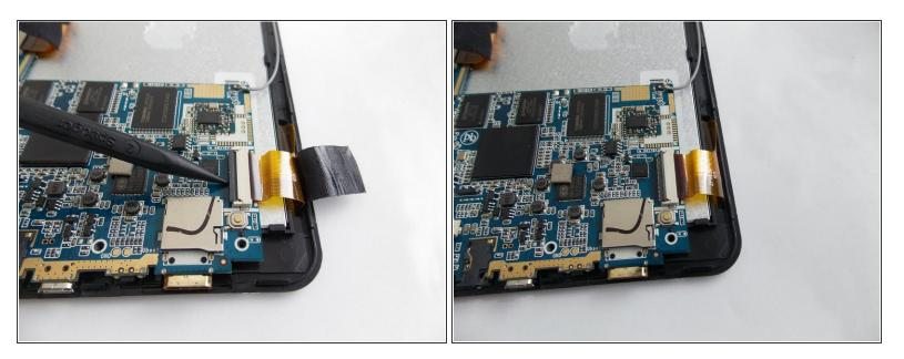
• Use the spudger tool to pry the ZIF connector upwards so that it releases the power cable.
