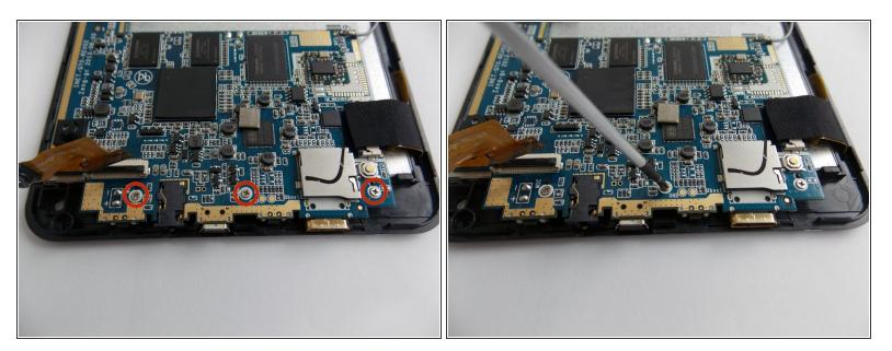
• Use the T4 Torx screwdriver to remove the 4.0 mm T4 Torx screws.
