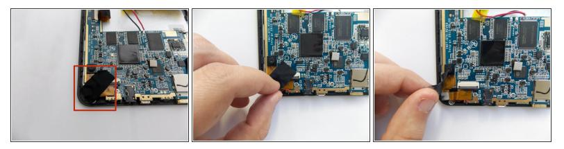
• Remove the black tape covering the cameras power cable.
