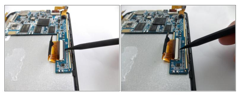
Use the spudger tool to pry the ZIF connector on the other side of the tablet upwards so that it releases the power cable.
