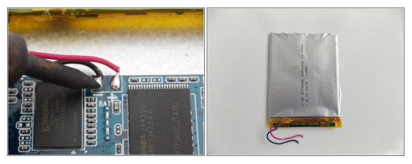
• Desolder the cables with a soldering iron and use a desoldering braid to remove the solder.
