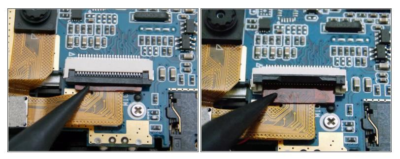
• Use the spudger tool to pry upwards the ZIF connector and release the power cable.
