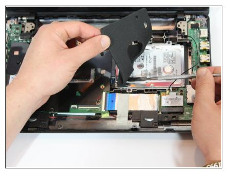
Remove the black foam and adhesive located on top of the hard drive.
