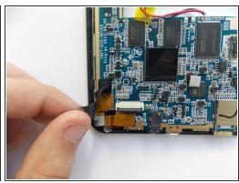
Remove the black tape covering the cameras power cable.
