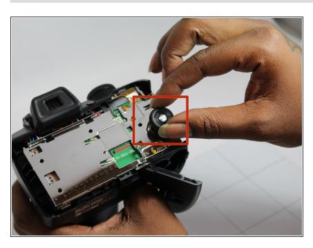
To Replace the Selection button, carefully pull the button until the button has been fully detached.
