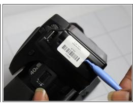
Carefully pry away the rear housing cover with the plastic opening tool.
