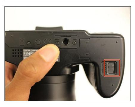
Push the battery chamber latch in the direction of the front of the camera. Keeping tension on the latch, slide the battery chamber cover toward the outside of the camera, opening the battery chamber.
