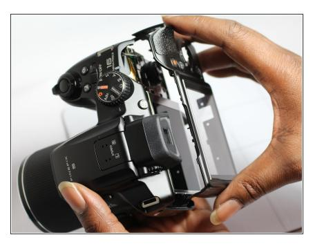
Remove the rear housing cover by carefully pulling it away from the camera.
