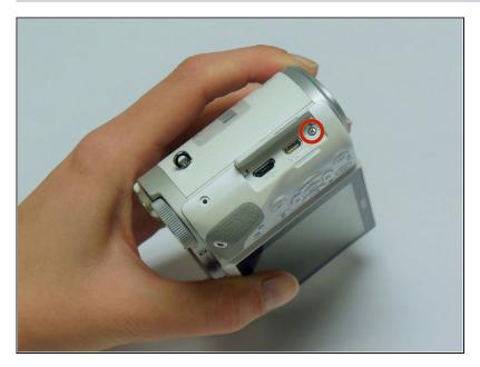
Using a Phillips #00 precision screwdriver, remove the last 4 mm screw located inside the input ports' compartment.
