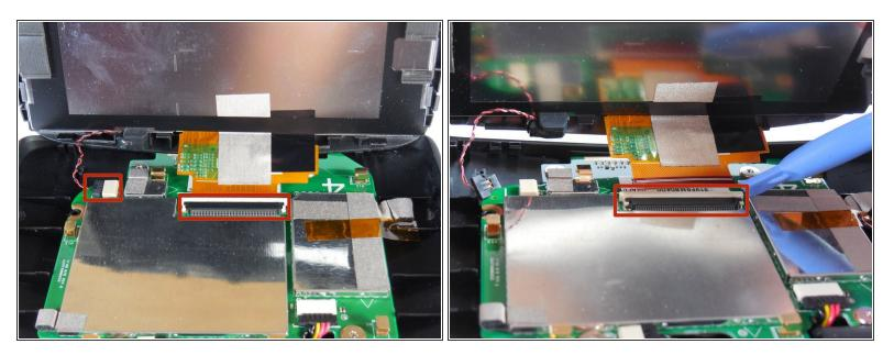
• Carefully remove the reset button cable (located on the left) and the ribbon cable.
