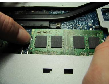
Gently pull apart clips on the ends of the memory module until the memory module pops up.
