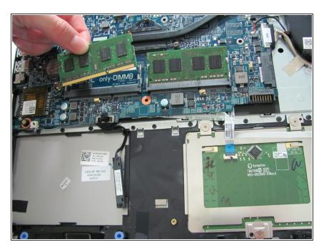
Pull the RAM out at a 45 degree angle.
