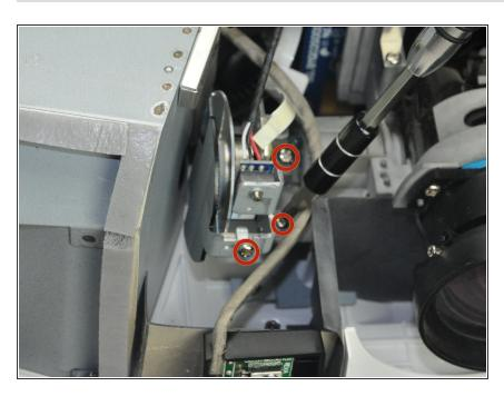
Use a Phillips #1 screwdriver to remove the 5.5 mm screws around the pin wheel.
