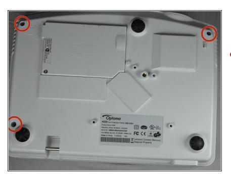
Use a Phillips #1 screwdriver to remove the three 7.5mm screws on the bottom of the device.
