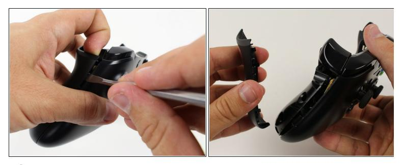
*i* We recommend using a nylon spudger for this step. A metal spudger is shown.
