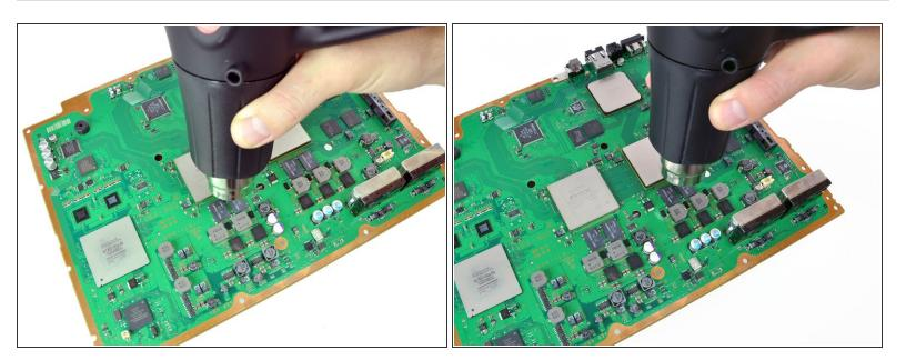
Continue heating the chips using the same circular motion as described above, for about 25 seconds each.
