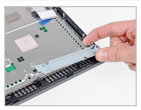
Remove the control board bracket.
