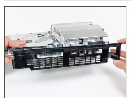
Remove the rear cover from the logic board assembly.
