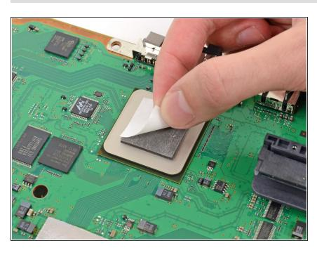
Peel the remaining white plastic cover off the other side of thermal pads.
