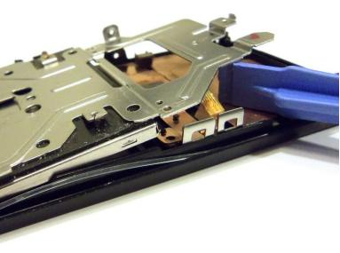
Pry the end of the screen with the plastic opening tool.
