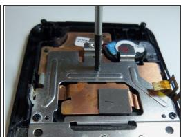
• Use Phillips size 00 and remove the 3 screws as shown.
