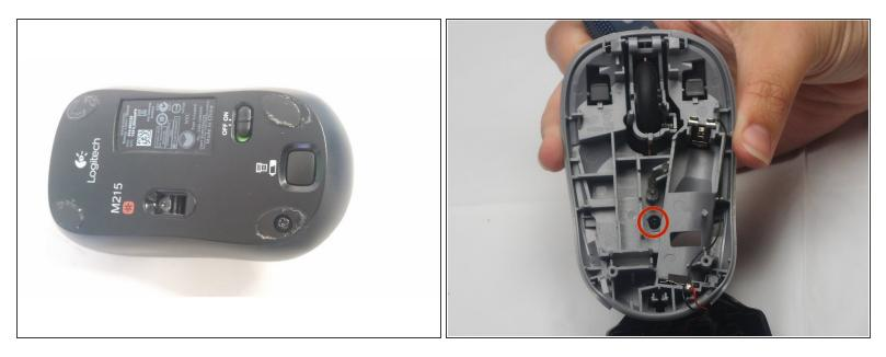
Use your fingernail to carefully remove the two skid stickers from the fat (non-button) end of the bottom of the mouse to reveal two Philips head screws. Remove these, then unclip the bottom cover. Don't get the sticky dusty. Now remove buttons; they're both attached by one 0.5mm Phillips head screw. It is located in the center of the top cover.
