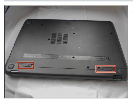
There are two battery release switches circled.
