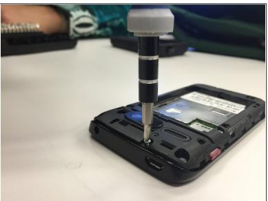
Remove seven of the 4.9mm tri-head screws. Keep them in a secure location.
