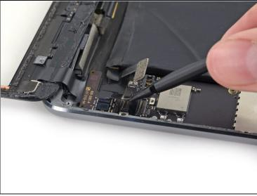
• Use the flat end of a spudger to lift the digitizer cable connector straight up off of its socket.
