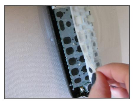
To better access the screen, remove the loose gel casing that sits under the keyboard.
