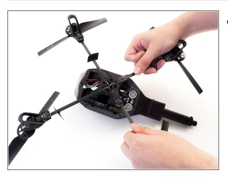
The central cross can now be removed and replaced.
