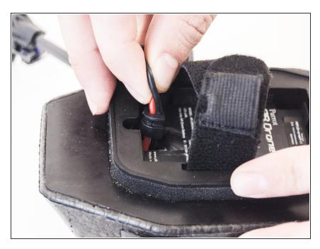
Release the rubber clip holding the USB and battery power cable to the body.
