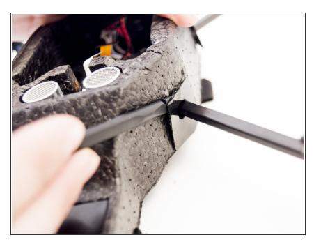
Using a nylon spudger, peel off the four pieces of plastic securing the frame to the body.
