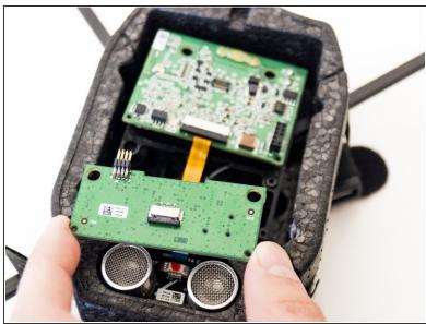
Carefully pull the secondary board from the mainboard.
