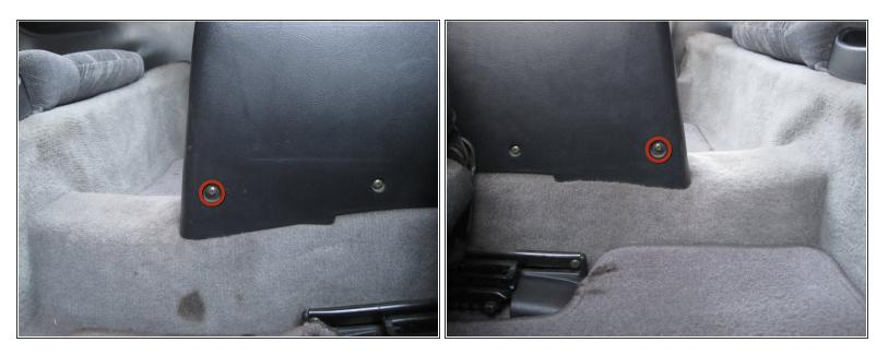
• Remove the two Phillips screws at the very rear of the center console near the floor.
