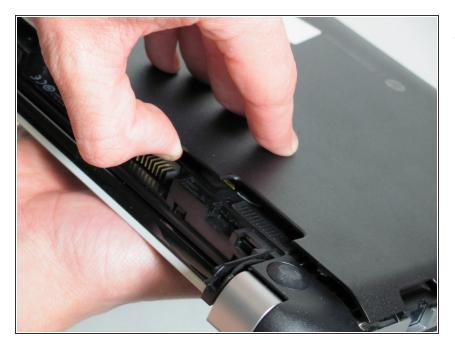
Using a spudger, pry the plastic plate off of the base of the computer.
