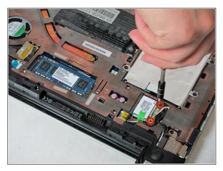
Remove the screws from the WLAN card
