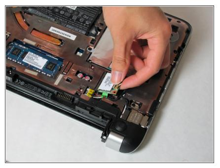
Remove the card by sliding out of the slot.
