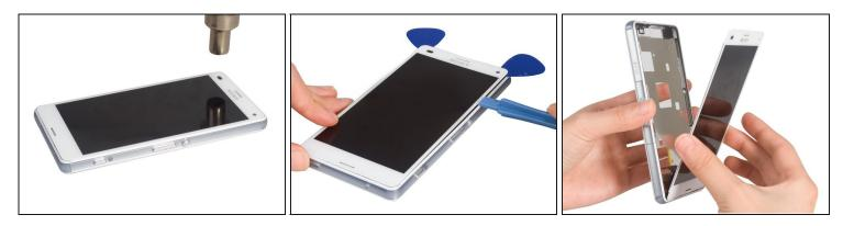
• Separate the LCD screen with earpiece from midframe. See the detail on <u>Sony Xperia Z3</u> <u>Compact LCD screen replacement guide</u>. Finally, you you can reassemble the phone with new midframe.
