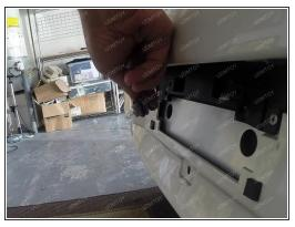
Pull out the license plate lamp assembly and remove the stock license plate bulb.
