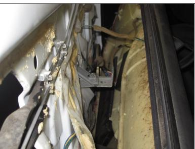
Pull the bottom of the door panel away from the door, and lift the entire panel off the door.
