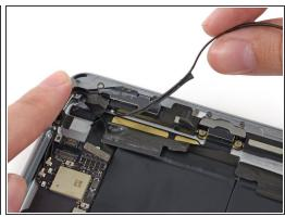
Lift the antenna cable tape up from behind the right speaker.
