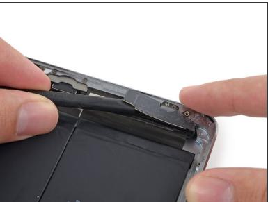
Use the flat end of a spudger to loosen the foam adhesive securing the Wi-Fi antenna to the left speaker.
