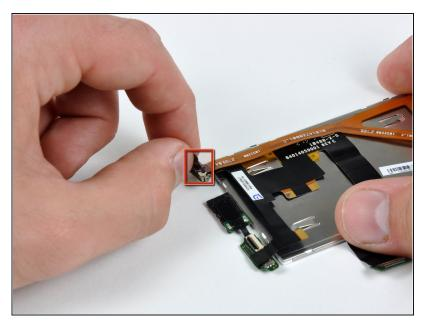
Peel away the black tape to reveal the display data cable connector.
