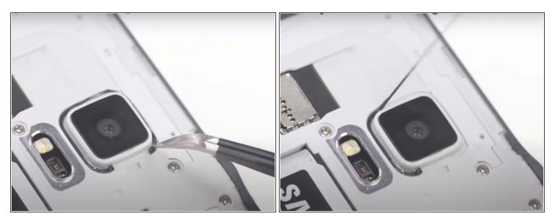
• Use a pair of tweezers to peel off the camera ring adhesive.
