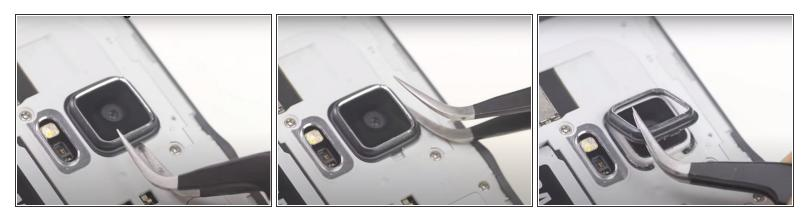
• Use a pair of tweezers to pry off the rear-facing camera ring.
