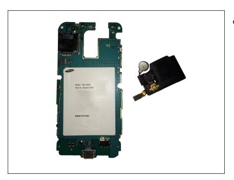
The speaker/rear camera has now been removed from the board.
