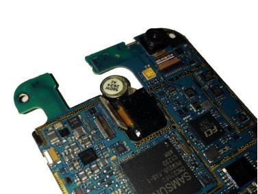
Flip the logic board to the rear side, and using a spudger/plastic pry tool to disconnect the rear camera flex cable.
