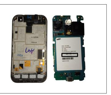
You have now removed the logic board from the display assembly.
