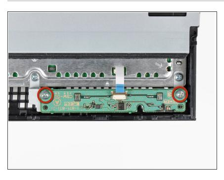
Remove the two 12 mm Phillips screws securing the control board to the lower case.
