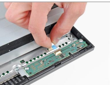
Use your fingernail to flip up the retaining flap on the control board ribbon cable socket.
