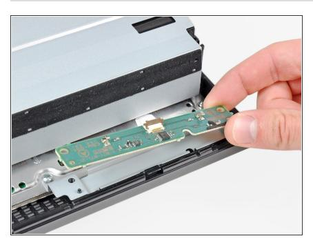
Remove the control board from the lower case.
