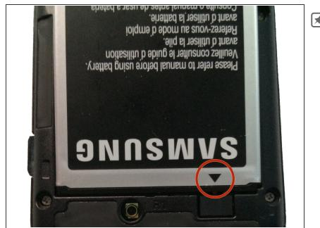
Make sure when replacing the battery that the arrow on the bottom is facing down.
