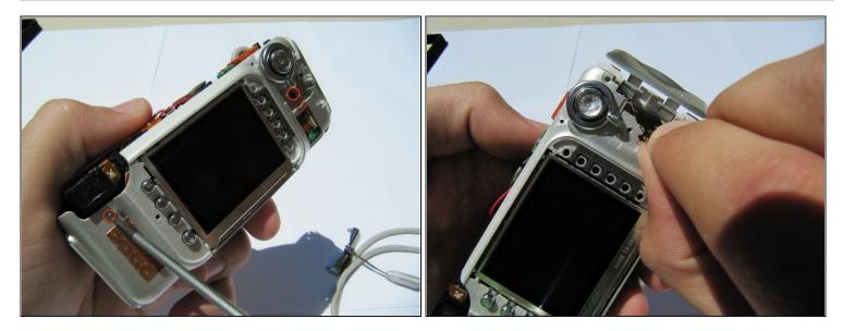
• Remove the back panel screws (1x 3.33mm, and 1x 3.40mm).
