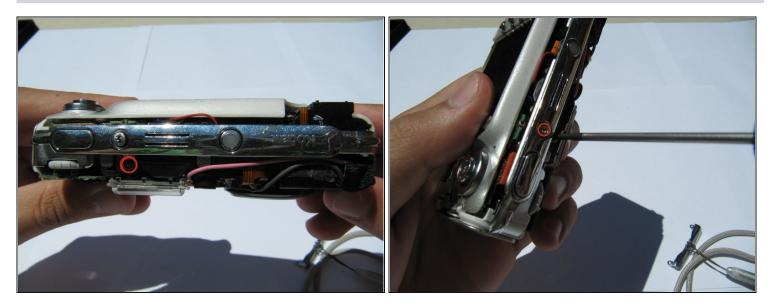
• Remove the top panel screw (1x 4.37mm).
