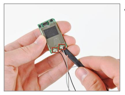
• Use the flat end of a spudger to pry both antenna connectors off their sockets on the Wi-Fi board.
