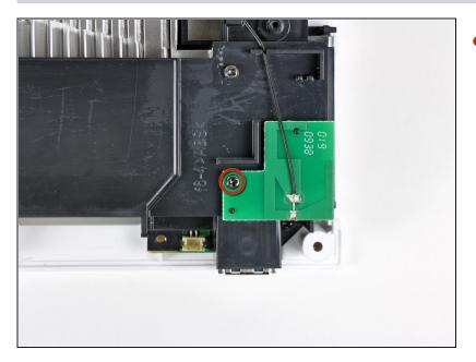
Remove the single 10 mm Phillips screw securing the second Wi-Fi antenna to the top of the fan shroud.
