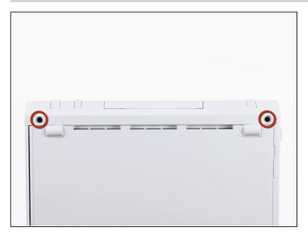
Remove the two 8.3 mm Tri-Point screws hidden under the covers you just removed.
